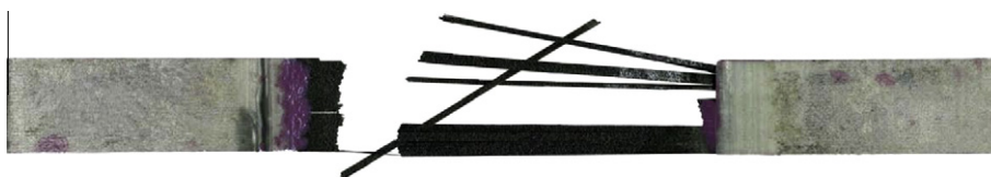
Fig. 5. Typical tensile failure for a coupon without defect.
