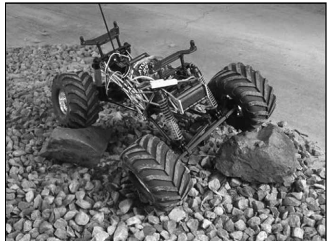
Figure 6. Reduced scale rover test bed for 12.7 cm diameter wheels.
