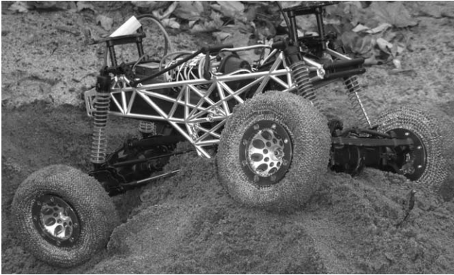
Figure 16. 12.7 cm diameter iRings wheels on reduced scale rover.
